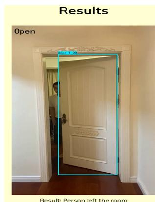
Figure 3. Door open detection.
